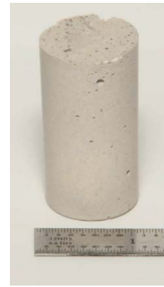
Figure D-11 Troy clay geopolymer monolith of Hanford LAW 60% FBSR product (Jantzen 2015)
