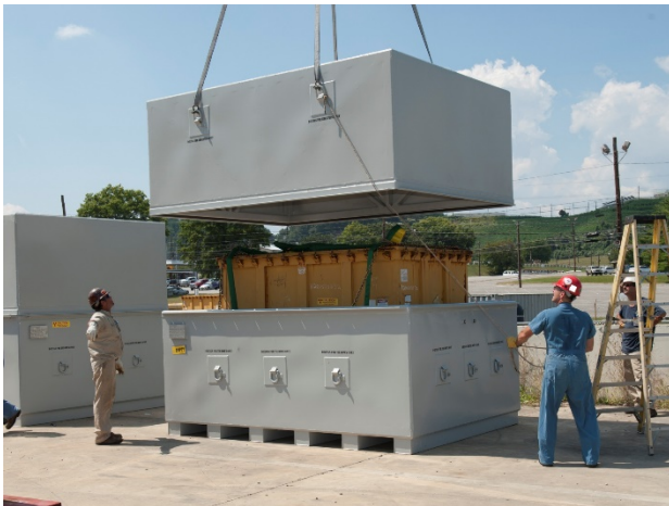
Figure G-3 Example of a Reusable Steel Split-Cavity Overpack (actual overpack would be smaller, lighter, and with a shallower lid) (photograph from Container Technologies Industries, LLC literature 122 )
